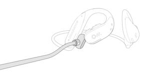
Connect the earphones' magnetic charging contact to the magnetic charging wire; the magnets will accurately align and optimize charging for the most efficient and stable position.
