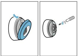
**2.** Open the cooking sensor lid and remove the battery from the base.
