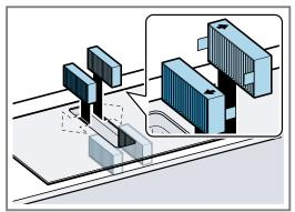
6. Insert the grease filter.
